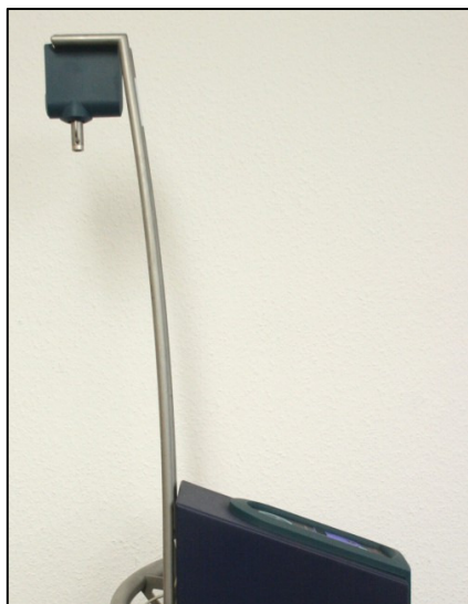
Fig. 13: la barre support correctement installée
